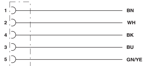
Contact assignment of the M12 sockets
