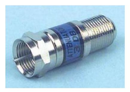
Nickel-plated, solid brass body, monolithic ceramic printed circuit board, ensuring rugged construction, etched glaze-type resistors provide  $\pm 5\%$  accuracy and excellent return loss, small 1.375" size, 22-gauge spring steel center pin, female to male fitting, not DC passive.
