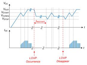
Figure 25. LOVP Waveforms
