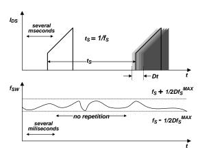
Figure 27. Frequency Fluctuation Waveforms
