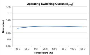
Figure 5. Operating Supply Current (I<sub>OP</sub>) vs. T<sub>A</sub>
