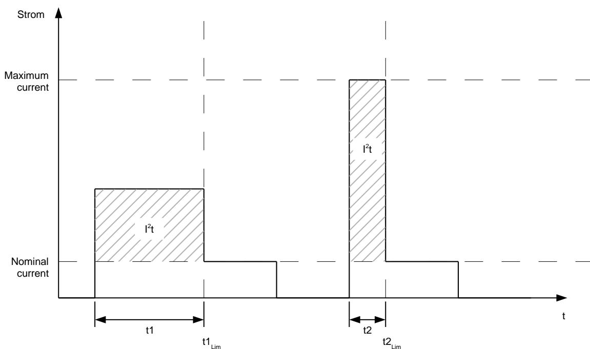
In the first section  $t_1$ , the current value is higher than the nominal current. At time  $t_{1,Lim}$ ,  $I^2t_{Lim}$  is reached and the current is limited to the nominal current. During the following time period  $t_2$ , a current comes that corresponds to the maximum current. Accordingly, the value for  $I^2t_{Lim}$  is reached faster than in time period  $t_1$ .
