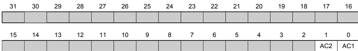
In general: If a bit is set to 0, the analog input measures the voltage; if the bit is set to 1, the current is measured.
