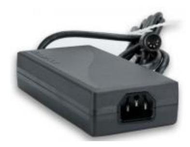
The PRO-S Power Supply is a UL approved triple output DC wall mount power adapter for use with the PRO-S-LAB. The PRO-S has input source: 100-240 VAC / 50-60 Hz, outputs of 5 VDC @ 2A, +12 VDC @ 1 A, -12 VDC @ 0.2 A. The output is provided through a 5-pin DIN connector.
