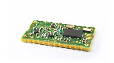
The **PE868-25mW Power Efficiency** is a RF transceiver which allows to implement data transmission over long distances while maintaining **very low power consumption**.
