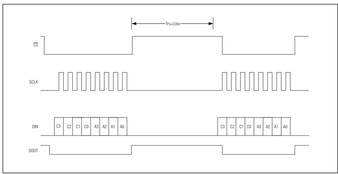
Figure 9. Manual Conversion Timing Without Reading Data
