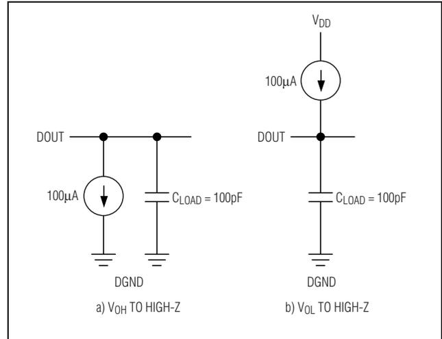
Figure 2. Load Circuit for DOUT Disable Time
