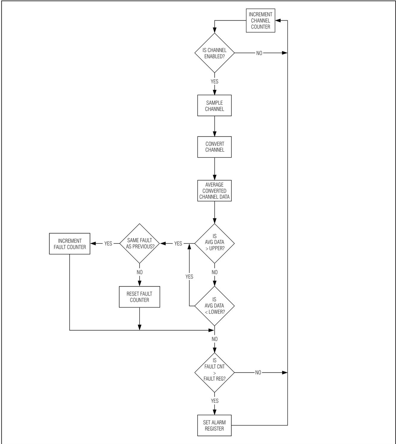
Figure 4. Alarm Flowchart
