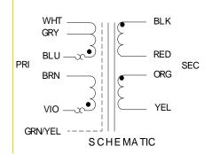
POWER TRANSFORMER CHASSIS MOUNT: TOROIDAL MEDICAL SERIES
