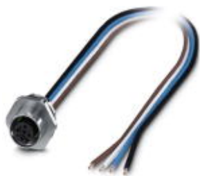
Flush-type connector, Universal, 4-position, SocketLink:M12, A-coded, Front mounting, M16 x 1.5, Individual wires, Cable length: 0.5 m
