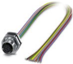
Flush-type connector, Universal, 17-position, SocketLink:M12, A-coded, Rear mounting, M16 x 1.5, Individual wires, Cable length: 0.5 m
