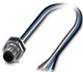
Flush-type connector, Universal, 5-position, PlugLink:M12, B-coded, Rear mounting, M16 x 1.5, Individual wires, Cable length: 0.5 m
