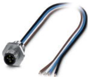
Flush-type connector, Power, 4-position, SocketLink:M12, T power, Front mounting, M16 x 1.5, Individual wires, Cable length: 0.5 m
