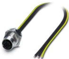
Flush-type connector, Power, 3-position, SocketLink:M12, S power, Rear mounting, M16 x 1.5, Individual wires, Cable length: 0.5 m
