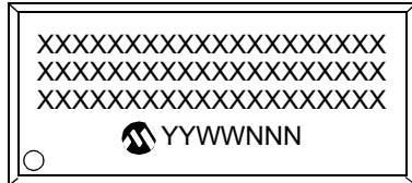
28-Lead UQFN (4x4x0.6 mm)
