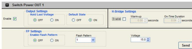
3. Under the Device Parameters section of this screen, set the default condition to "start up." This configures this Switch Power (Switch Power OUT 1) terminal to output continuous voltage as soon as the radio powers up.
