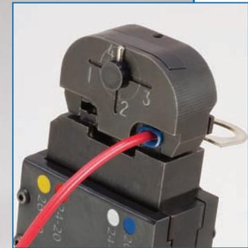
The height of the insulation crimp barrel can be adjusted to accommodate different insulation diameters.
