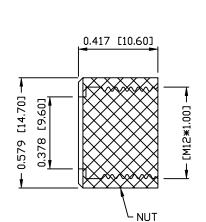
M12 FEMALE - CABLE MOUNT - SOLDER CUP - 3 POS.
