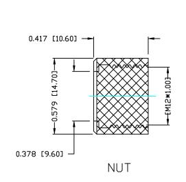
M12 FEMALE - CABLE MOUNT - SOLDER CUP - 5 POS.
