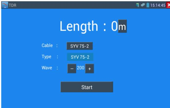
Built-in BNC cable, network cable, RVV control cable, Telephone line and TVVB cable etc can test. 11 groups user-defined cable can be set.
