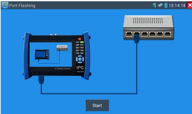
If the tester and PoE switch are connected well, the LAN port of POE switch flash at special frequency,
