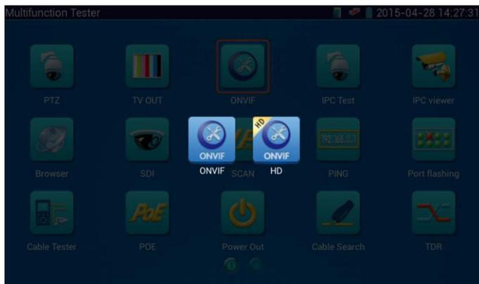
If you select ONVIF SD or HD mode, the meter automatically scans different network segments for ONVIF cameras. It lists the camera name and IP address on the Device List. If no cameras appear under
