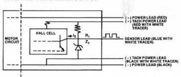
$I_{\rm S}$  = The sink capability of the collector of the hall cell = 15 mA maximum. R<sub>1</sub> and Z<sub>1</sub> are added to Tachometer Output fans to produce a fixed amplitude of VOUT.
