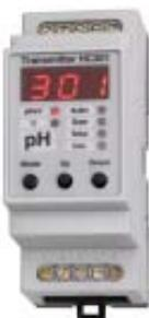
HC301 is a pH transmitter with 1 analogue output and it may be connected to a MODBus network for datalogging. Automated temperature compensation is possible using a Pt100/Pt1000 sensor or a fixed user selectable temperature. The unit displays pH and temperature (°C).
