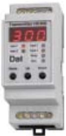
HC300 is a datalogger and MODBus master. The unit has 4 analogue inputs which may be logged. Furthermore up to 14 nodes may be connected using RS485, resulting in up to 60 measuring points. Sample times from 1 to 600 sec. Memory is 4 Mbyte FLASH
