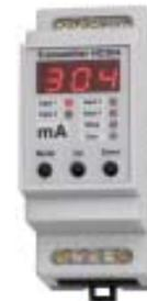
HC304 is a multipurpose transmitter with up to 4 analogue inputs. The unit has an analogue output and it may be connected to a MODBus network for datalogging. The measured inputs may be displayed as engineering values using the build-in scaling functionality.
