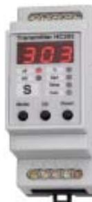
HC303 is a conductivity transmitter. The unit has 1 analogue output and it may be connected to a MODBus network for datalogging. Up to 3 measuring ranges may be selected. Auto. temperature compensation is possible using a Pt100/Pt1000 sensor. The unit displays conductivity and temperature.
