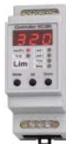
HC320 has two independent limits each free programmable as either max- or min-limit. The necessary timers (start- and response) and features needed for an efficient controller is also included. Input signal is any 0(4)-20mA and two relays signal alarm condition. The input signal may be scaled down to 50%.
