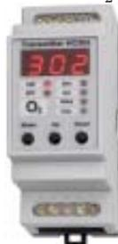
HC302 is an oxygen transmitter. It is produced in 2 versions depending on the oxygen sensor. The unit has 1 analogue output and it may be connected to a MODBus network for datalogging. Temperature-compensation is done using a Pt100 or an NTC sensor. The unit also displays temperature.
