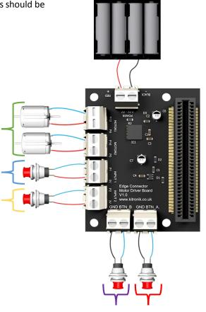
Pushing this button brings the BTN\_B pin low (0) and releasing it activates the 'button is pressed (B)' function in the code.
