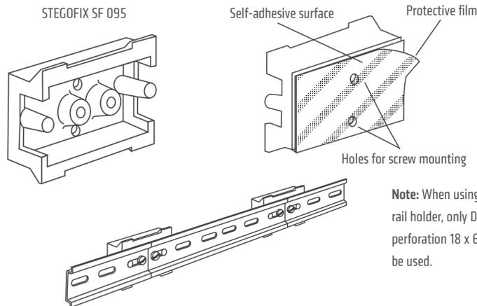
**Note:** When using the STEGOFIX as a DIN rail holder, only DIN rails (EN 60715) with perforation 18 x 6.2mm or 18 x 5.2mm can be used.
