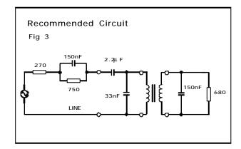
In practice, the 600Ù load resistor will connect to a low output impedance TX driver. The 150nF capacitor should appear in parallel with the 680Ù load resistor (rather than in parallel with transformer winding) to obtain optimum TX flatness to line.
