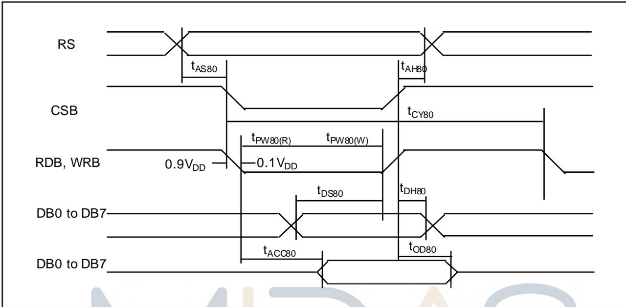
Figure 1. Read / Write Characteristics (8080-series MPU)
