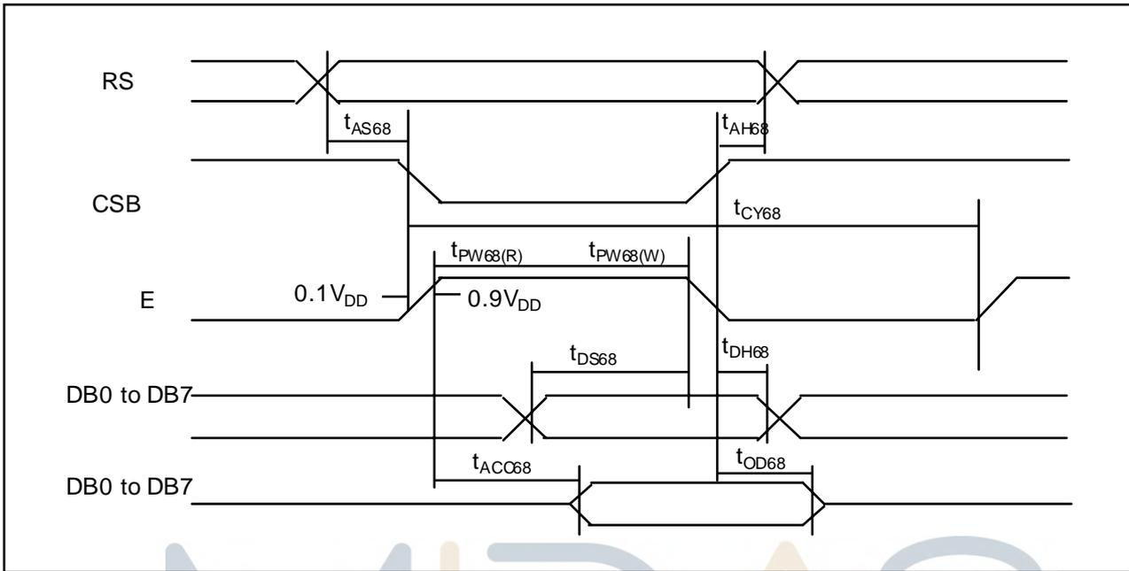
Figure 2. Read / Write Characteristics (6800-series MPU)
