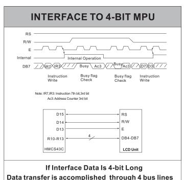
from DB4 to DB7.(while the rest of 4 bus lines from
