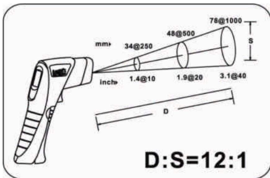
Approximate examples of distance to spot are shown in the diagram above. At a distance of 12 inches the spot diameter will be 1 inch.
