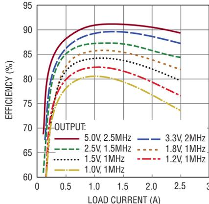
**Efficiency vs Load Current at 3.3V<sub>IN</sub>**
