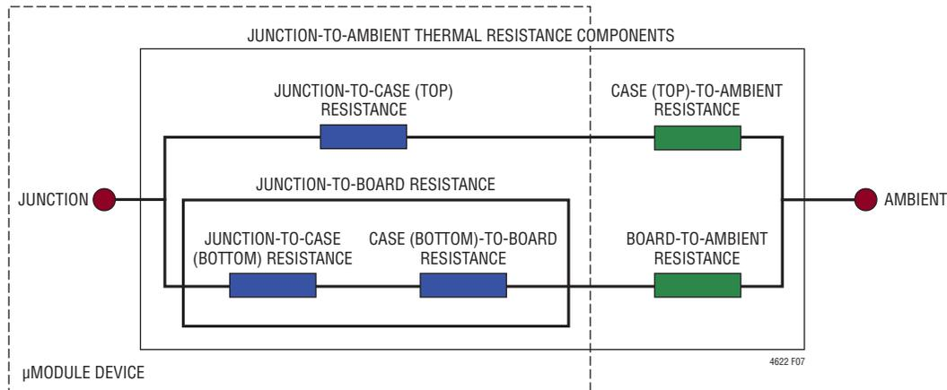
Figure 7. Graphical Representation of JESD 51-12 Thermal Coefficients
