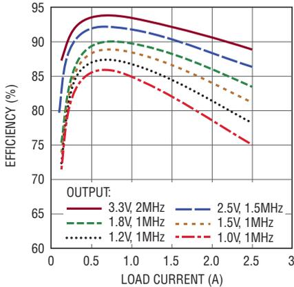
**Efficiency vs Load Current at 12V<sub>IN</sub>**
