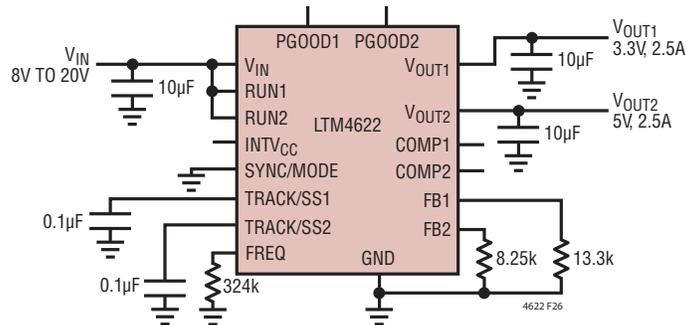
Figure 26. 8V<sub>IN</sub> to 20V<sub>IN</sub>, 3.3V and 5V Output at 2.5A with 2MHz Switching Frequency
