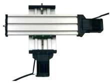
Of solid aluminium (surface-compacted), as described at right. With two step motors for the axes X (transverse) and Y (lengthwise). Table size and travel distances, see description of MF 70/CNC-ready.
