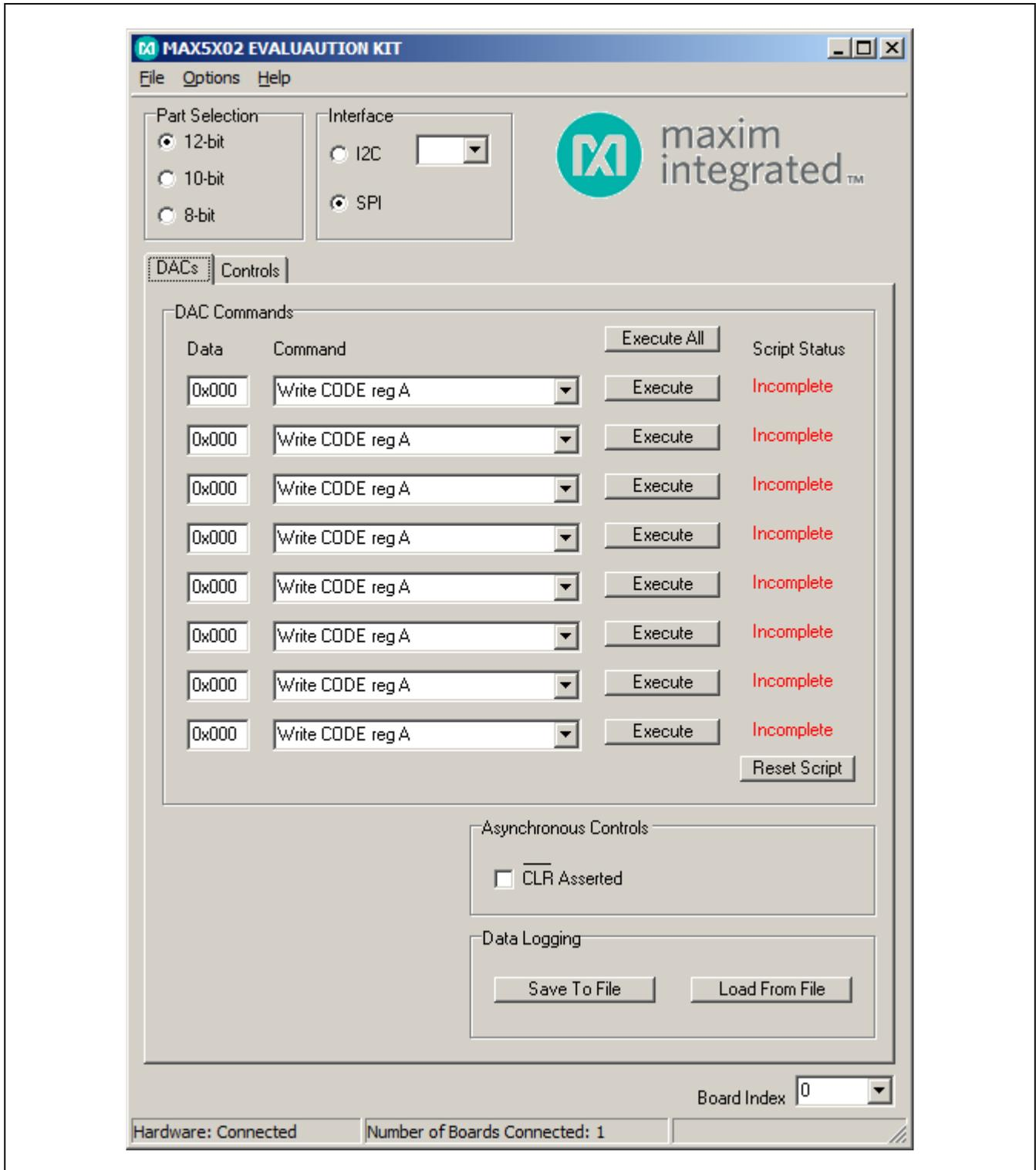
Figure 1. MAX5X02 EV Kit Software Main Window (SPI)
