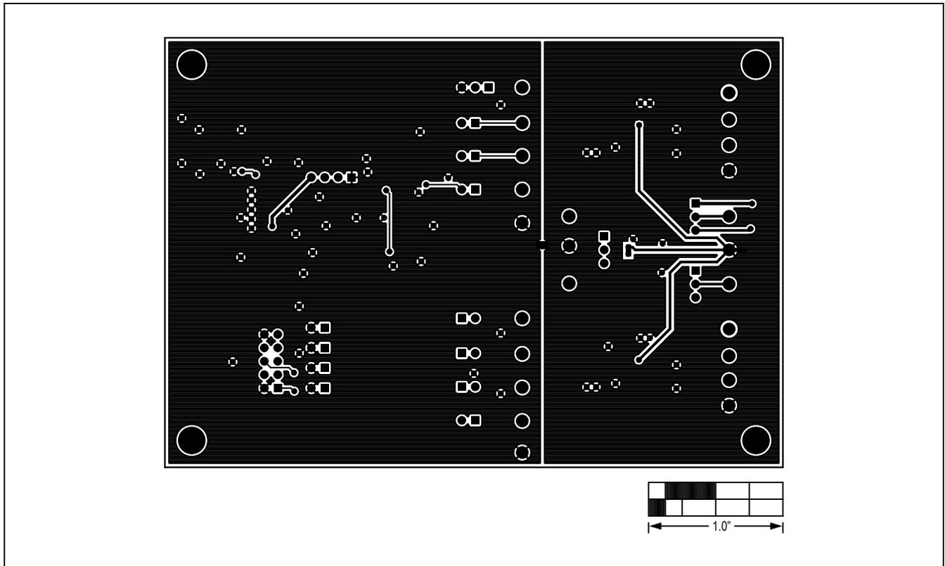
Figure 8. MAX5X02 EV Kit PCB Layout—Solder Side
