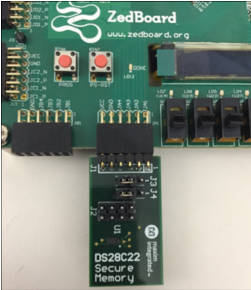
Figure 3. The MAXREFDES43# subsystem design correctly inserted into the ZedBoard development platform. Note that the MAXREFDES43# board is plugged into the top row of the Pmod connector on the ZedBoard.
