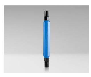
The SSK-716 can wrench is specifically designed to work with our SSK-85 and SSK-75 star keys. The SSK-716 can wrench has two 7/16" hex sockets 1 ½" deep on either end and can be used to open enclosures that require a 7/16" socket. With the SSK-75 and SSK-85 star keys you can open enclosures requiring any of the following star key patterns:
