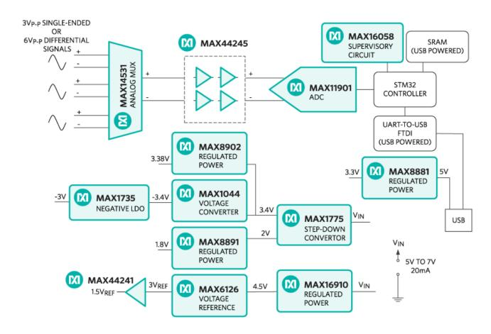
Figure 1. The MAXREFDES38# reference design block diagram.
