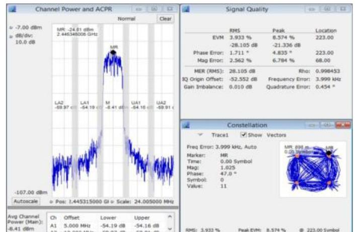
SignalVu-PC application SV26 enables quick, standards-based transmitter health checks on APCO P25 signals. The following image shows a Phase II signal being monitored for anomalies with the spectrum analyzer while performing transmitter power, modulation and frequency measurements.
