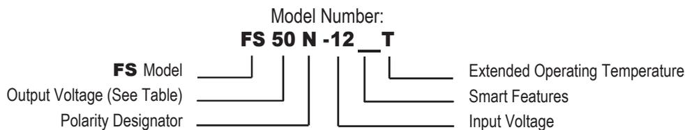
EXAMPLE: **FS50N-12T** (**FS**-Series, **50** - Output Voltage, **N** - Negative, **12** - Input Voltage, **Blank** - with Smart Features, **T** - Extended Operating Temperature)
