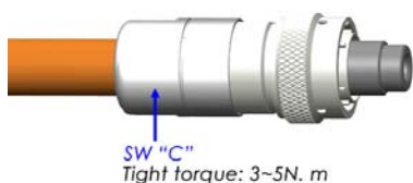
Step 9: Attach and tighten backshell as shown
