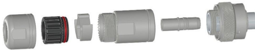
Step 1: Slide parts onto cable
