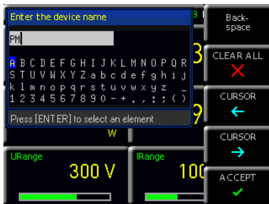
Fig. 9.4: Entering the instrument name.
