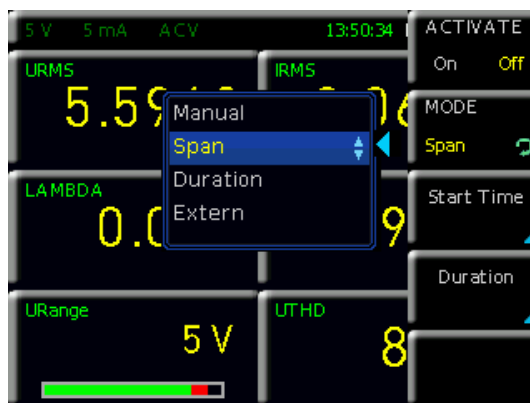
Fig. 6.12: Span integration mode selection menu.
