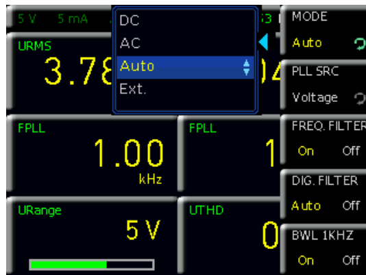
Fig. 6.15: Selecting the data acquisition mode.
