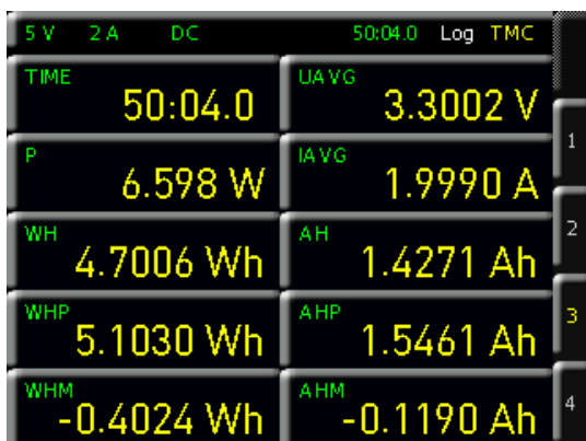
Fig. 6.10: Readout display with integrator output values.
