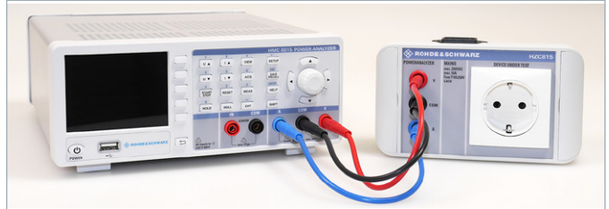
Fig. 4.1: Connecting HZC815 DE version to R&S®HMC8015.
