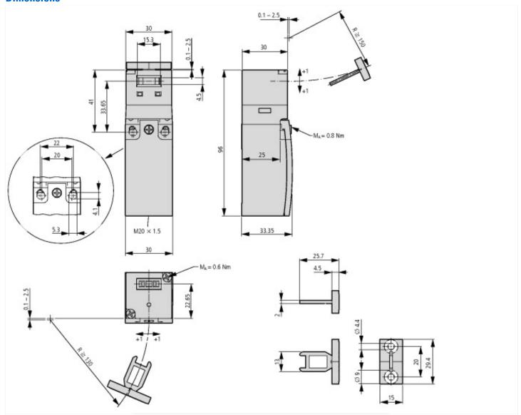
Switch must not be used as a mechanical stop Terminal marking according to EN 50 013 Travel [mm]
