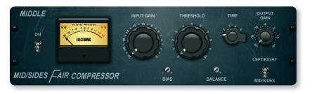
Our FAIR COMPRESSOR model is true to the original signal path, and conveniently provides models for dual, stereo-linked or M/S operation. (Inspired by Fairchild 670\*)
