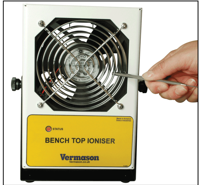
Figure 6. Shorting the ioniser fan grill to enclosure with a metal probe to test the alarm
