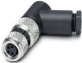
Connector, 4-position, Socket angled M8, A-coded, Screw connection, Knurl material: Nickel-plated brass, External cable diameter 3.5 mm ... 5 mm
