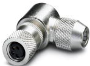
Connector, 4-position, shielded, Socket angled M8, A-coded, Solder connection, Knurl material: Nickel-plated brass, External cable diameter 3.5 mm ... 5 mm
