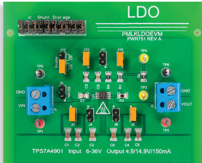
Figure 6. TPS7A4901 LDO board: jumpers set-up for Test#1
