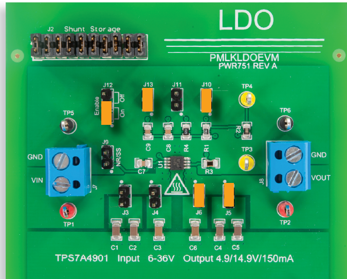
Figure 7. TPS7A4901 LDO board: jumpers set-up for Test#2
