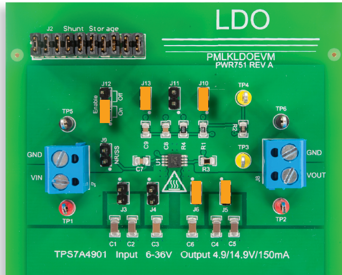
Figure 6. TPS7A4901 LDO board: jumpers set-up for Test#1
