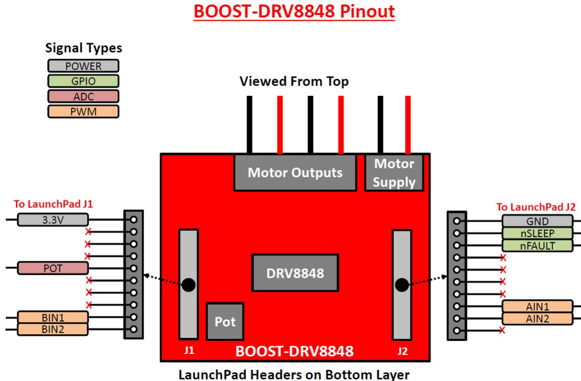
**Figure 4. BOOST-DRV8848 Pinout**
