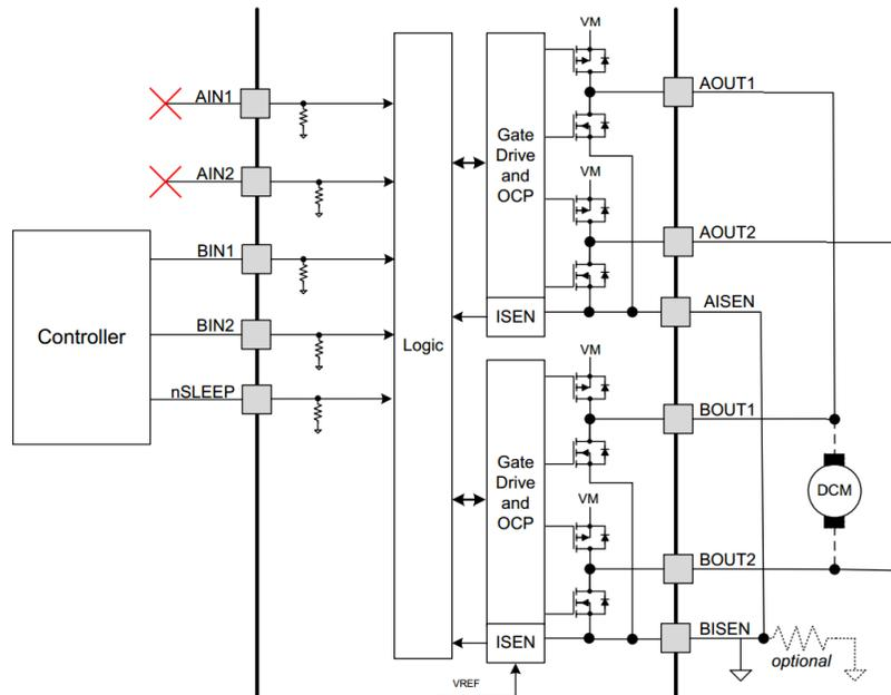
**Figure 16. Parallel Mode Operation**
