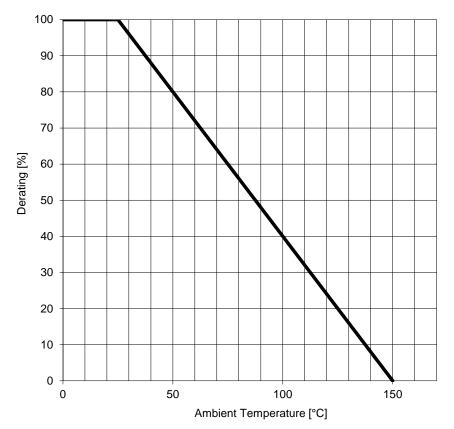
**Steady State Power Dissipation Derating:**
