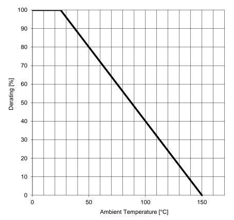
**Steady State Power Dissipation Derating:**
