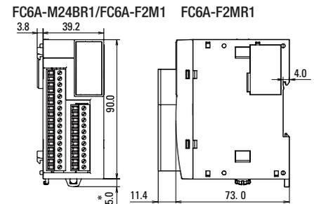
\* 9.3 mm when the clamp is pulled out.
