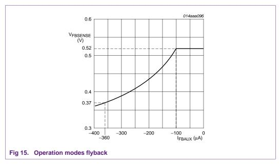
See <u>Figure 14</u>, the total OPP resistance determining the I<sub>FBAUX</sub> current during the primary stroke of the flyback exists of R23 + R23A. First, the OVP resistor R23 has to be calculated before the remaining part of the OPP resistor R23A can be calculated.
