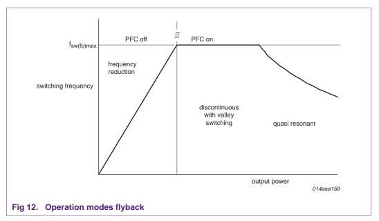
At maximum output power, limited by the flyback current sense resistor, the flyback operates in Quasi Resonant (QR) mode. The next primary switching cycle starts at detection of the first valley.
