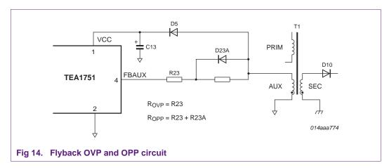
At a current  $I_{ovp(FBAUX)}$  of 300  $\mu A$  into the FBAUX pin, the IC detects an overvoltage. An internal integrator filters noise and voltage spikes. The output of the integrator is used as an input for an up-down counter. The counter has been added as an extra filter to prevent false OVP detection, which might occur during ESD or lightning events.
