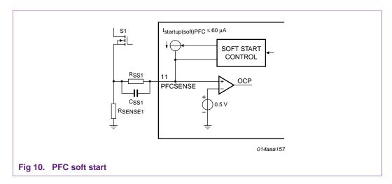
The total soft start or soft stop time is equal to:  $t_{softstart} = 3Rss1 \cdot Css1$
