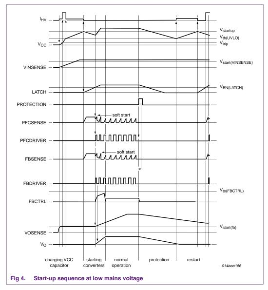
The charge time of the soft start capacitors can be chosen by their values independently for the PFC and the flyback. This way it can be realized that the PFC starts before the flyback.
