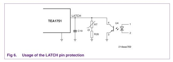
Latching on application over temperature occurs when the total resistance value of the NTC and its series resistor drops below the following:
