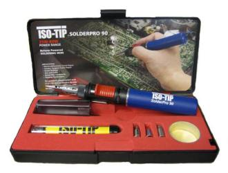
Pro 90 Soldering Iron/Torch Kit (#9010) The multi-Purpose Soldering Iron Kit is butane powered and can be easily carried and used anywhere. The unit has adjustable tip temperatures ranging in 480°F to 1,000°F. A single refill allows up to 55 minutes of continuous use.
