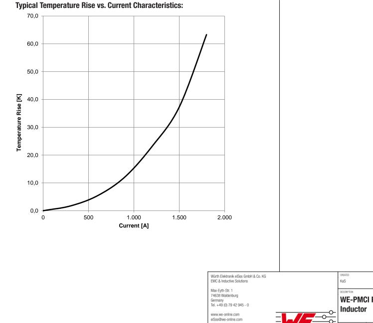
GENERAL TOLERANCE PROJECTION METHOD CHECKED DDi DIN ISO 2768-1m **WE-PMCI Power Molded Chip** ORDER CODE 74479276222C REVISION STATUS DATE BUSINESS UNIT PAGE 001.000 Draft 2016-04-14 3/6 eiSos 0806 WÜRTH ELEKTRONĬK
